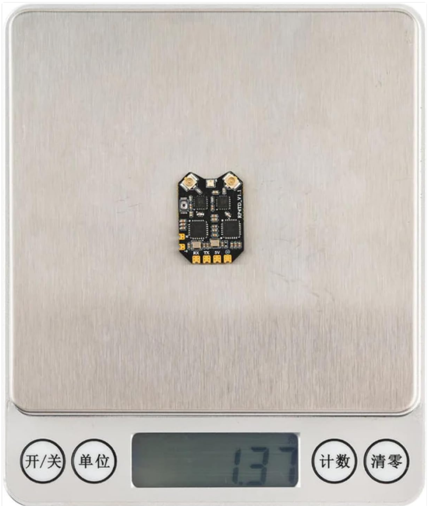
Image: The RP4TD receiver board placed on a digital scale, indicating a weight of 1.37 grams, highlighting its lightweight design.
