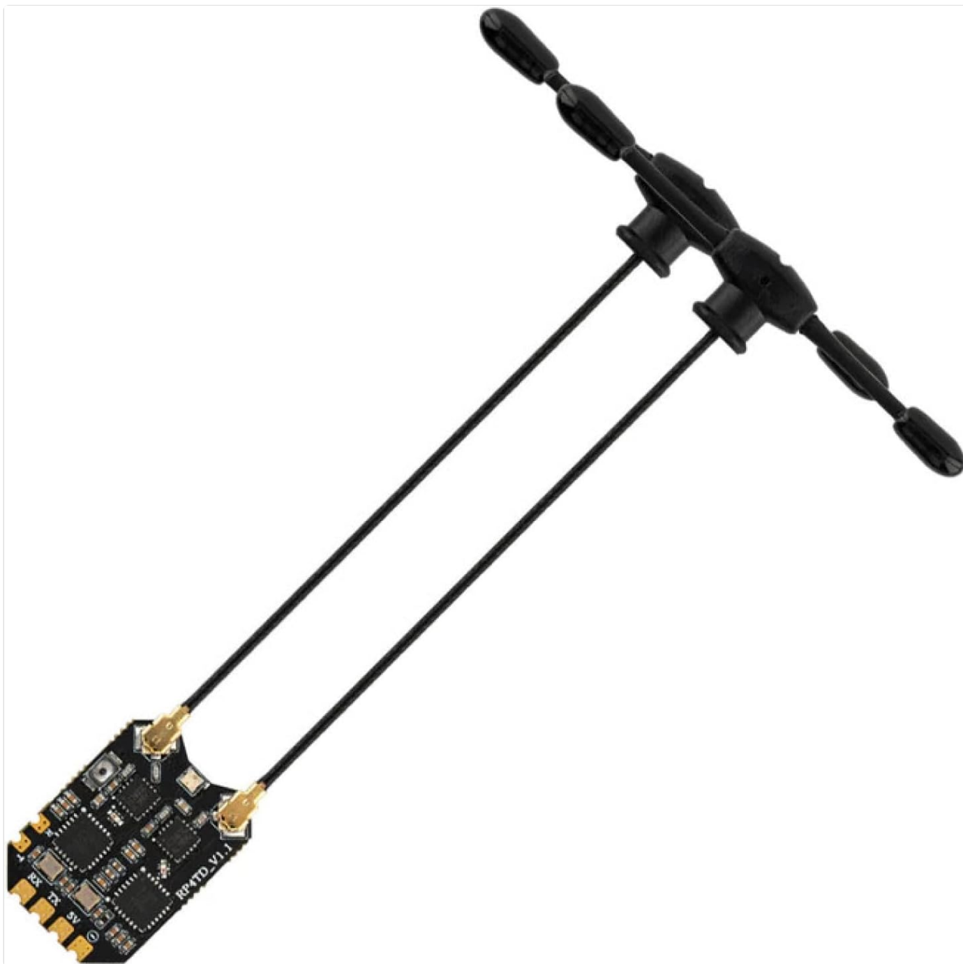
Image: The RadioMaster RP4TD receiver fully assembled with its two 65mm UFL T antennas, showcasing its compact design and dual antenna setup for diversity reception.
