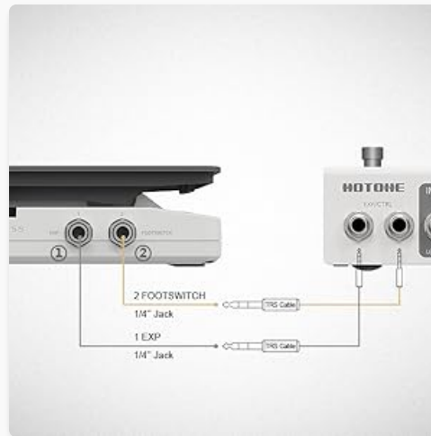
Image: A diagram illustrating the correct wiring for the Ampero II Press. It shows the EXP output connected via a TRS cable and the FOOTSWITCH output also connected via a TRS cable to a multi-effects unit, indicating the need for TRS cables for both functions.
