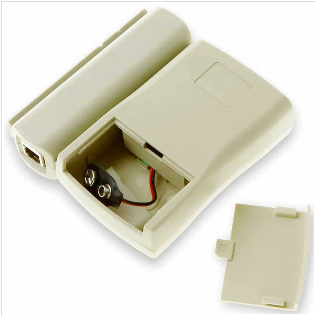
Figure 3: Rear view of the ITGlobal BS-468 Network Cable Tester, showing the battery compartment for a 9V PP3 battery.
