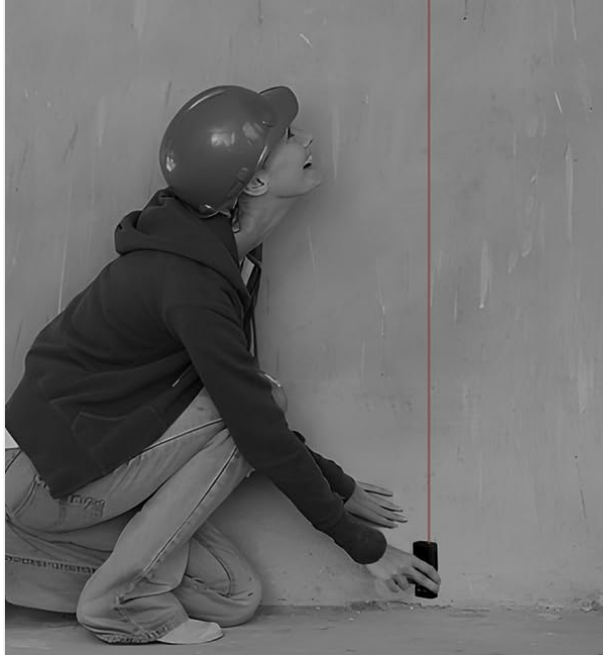
Figure 6.1: The dual laser system measures distances in two directions from the device's position.
