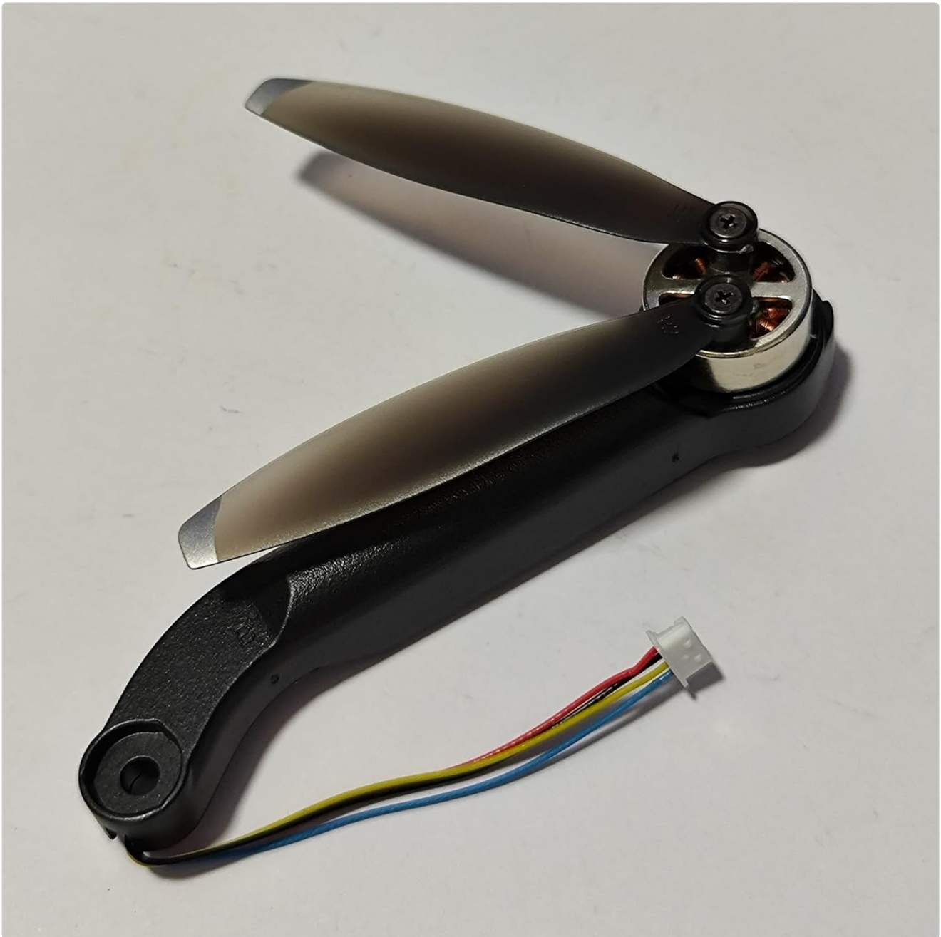
Image 2: DAYUDDRICAR KF613 Drone Rear B Motor Arm. For reference, this image displays a Rear B motor arm, which differs in orientation and wiring from the Front B arm.
