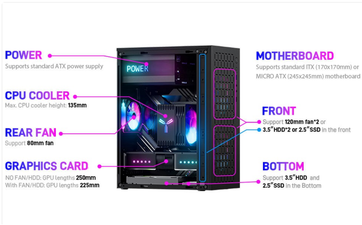
Figure 3: Detailed Case Dimensions
