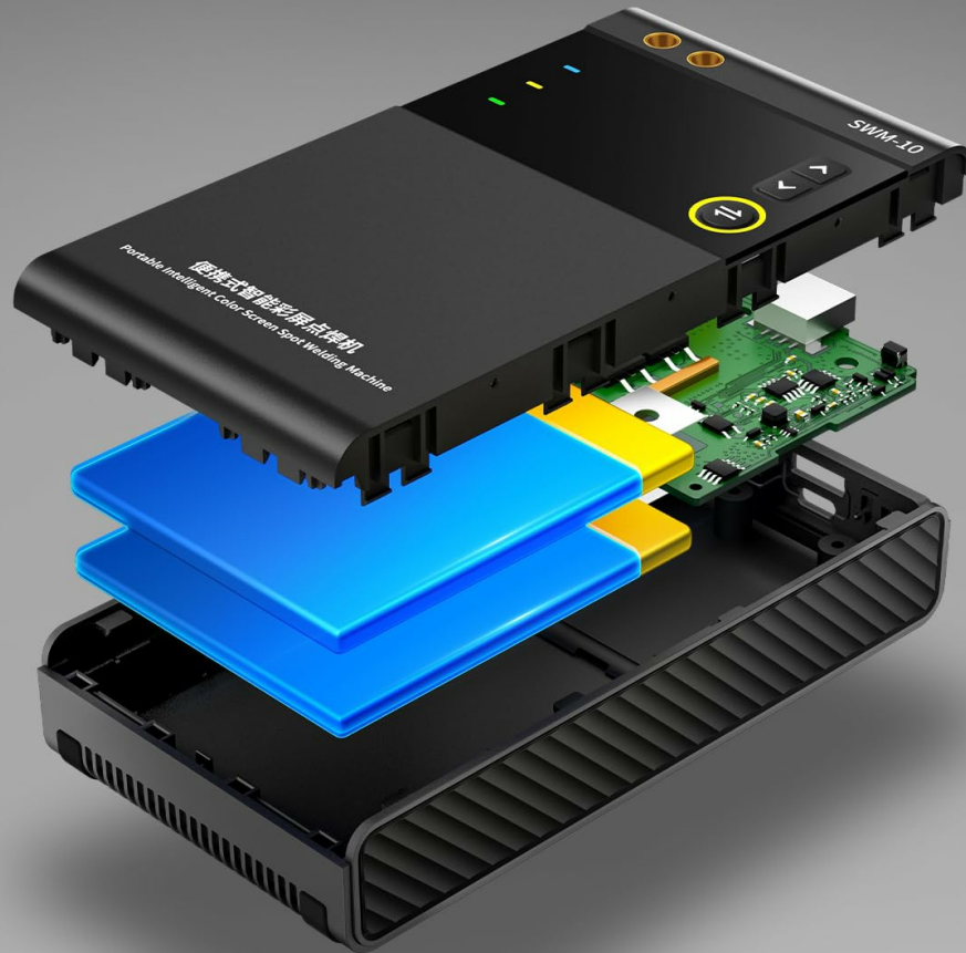
Figure 3.3: Internal components of the FNIRSI SWM-10, showcasing the high-quality A-grade batteries.
