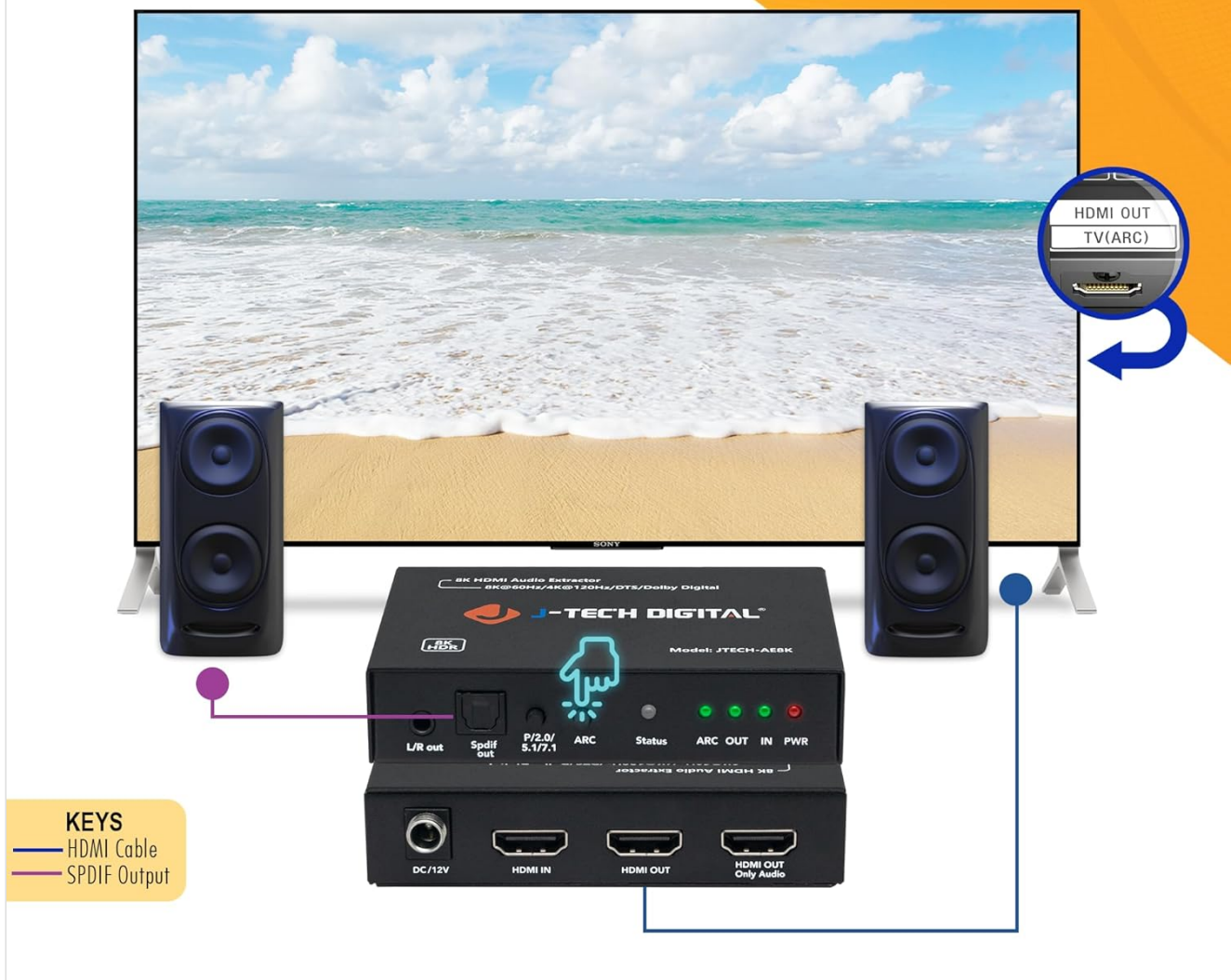
Image 6.1: Diagram explaining the ARC function and its audio routing.
