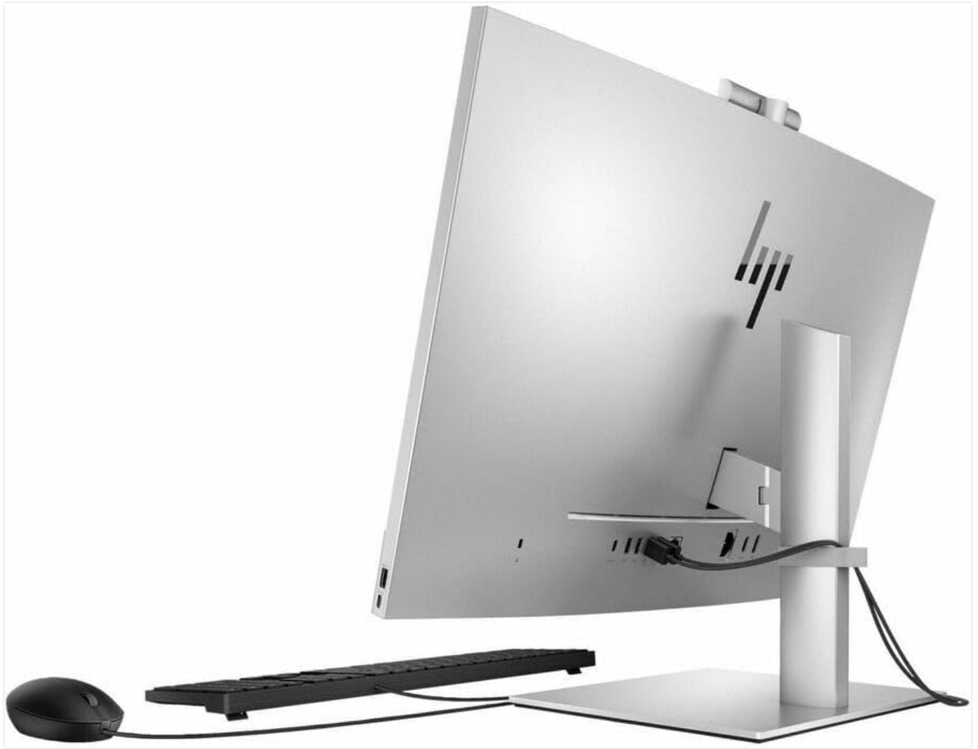
Figure 2: Rear ports of the HP EliteOne 870 G9 AiO PC. Connect your keyboard and mouse here.
