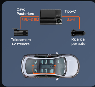
Image: Illustration of the dash cam and rear camera installation process, showing cable routing.
