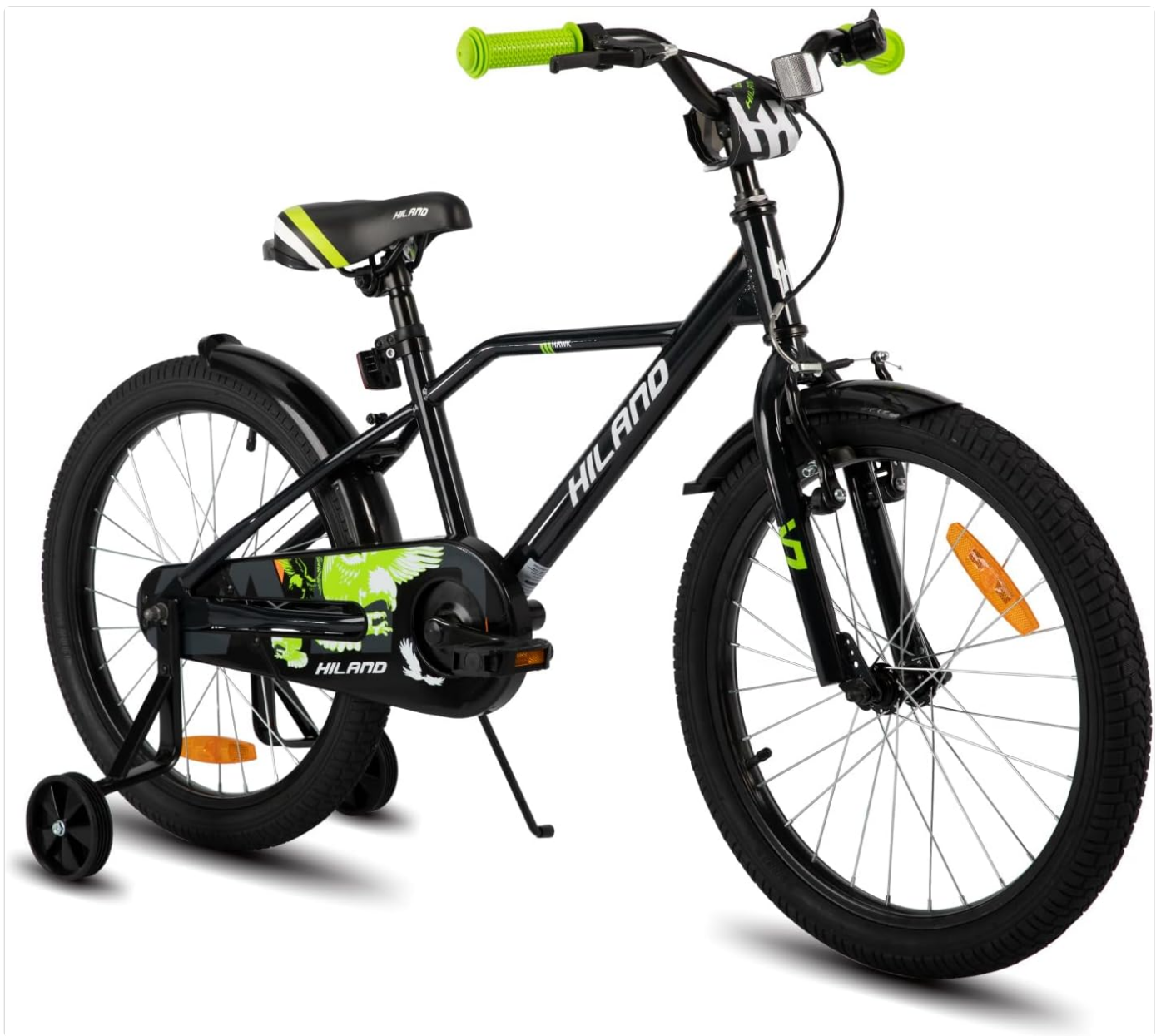
Figure 1: Overview of the HILAND 20 Inch Kids' Bicycle. This model comes equipped with training wheels, a hand brake, and a coaster brake, making it suitable for young riders.
