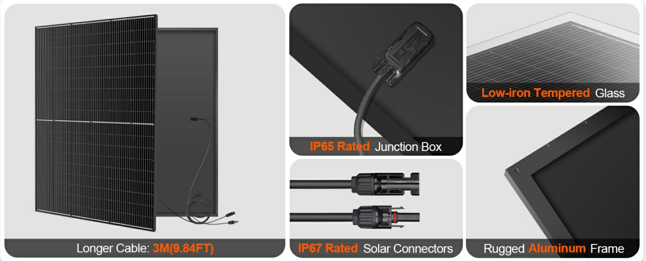
Image 3.2: Key components include low-iron tempered glass for optimal light transmission, an IP65 rated junction box for protection against dust and water, IP67 rated solar connectors for secure and waterproof connections, and a rugged aluminum frame for structural integrity.
