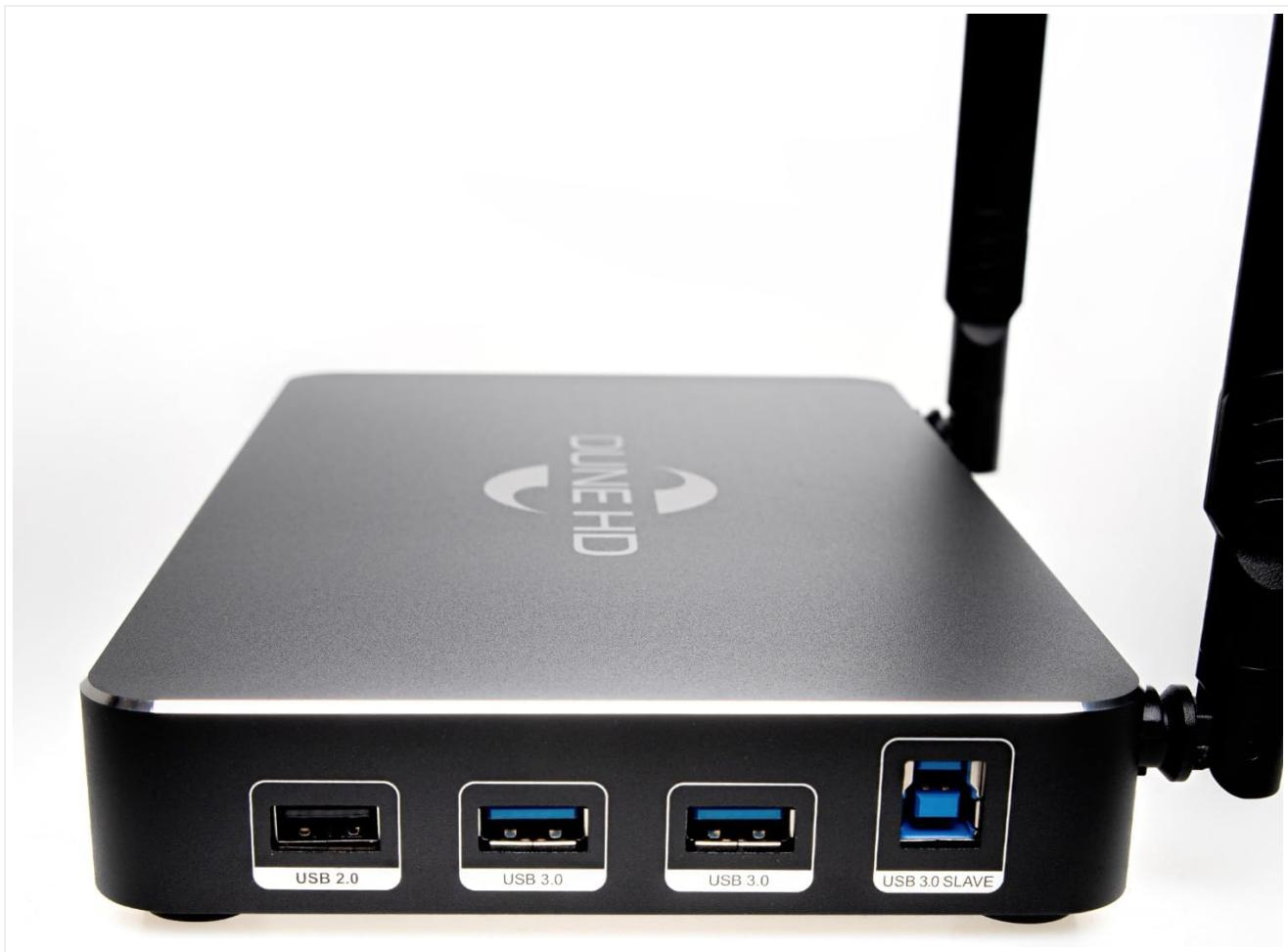
Side panel connections: USB 2.0, two USB 3.0 ports, and a USB 3.0 Slave port for PC connection.
