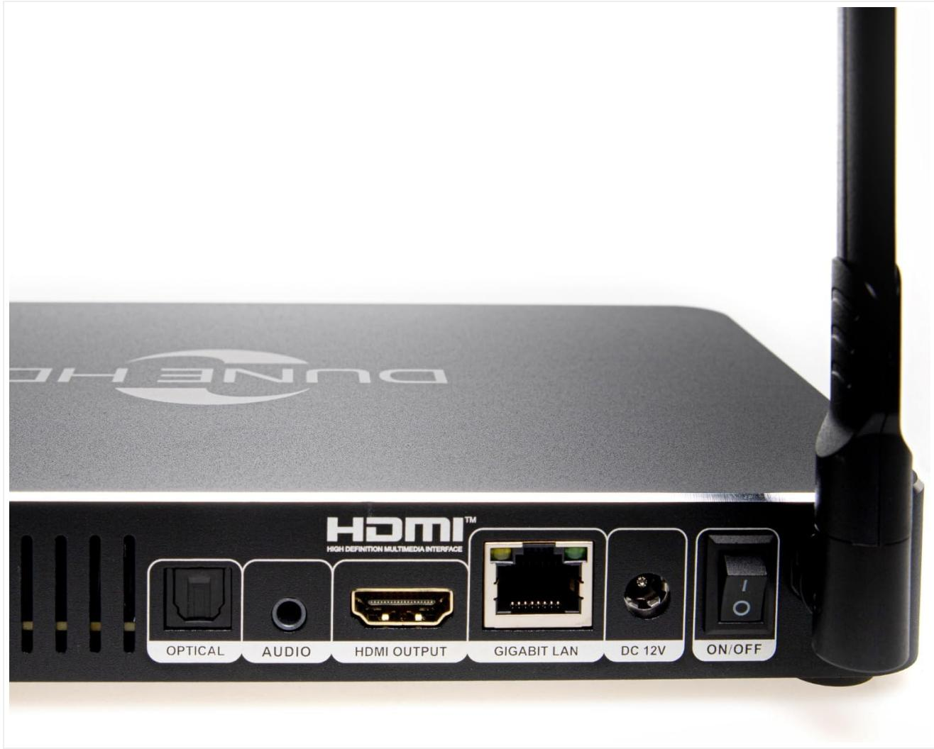
Rear panel connections: Optical audio, analog audio, HDMI output, Gigabit LAN, DC 12V power input, and power switch.
