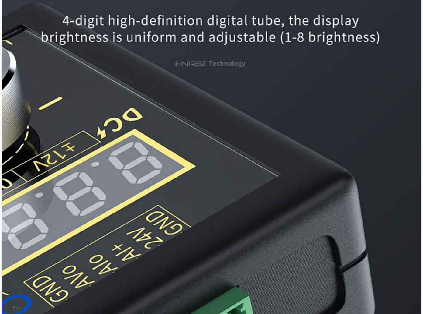
Figure 3.2: Detail of the display and pluggable terminals.
