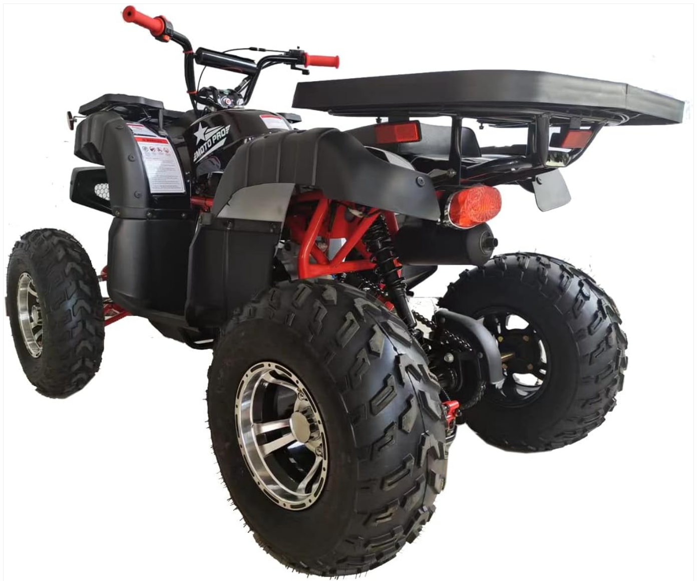
Figure 2.3: Rear view of the X-PRO Jaguar 200 ATV. This image shows the tail light, exhaust system, rear disc brake, and the large rear wheels. The rear cargo rack is prominently featured.
