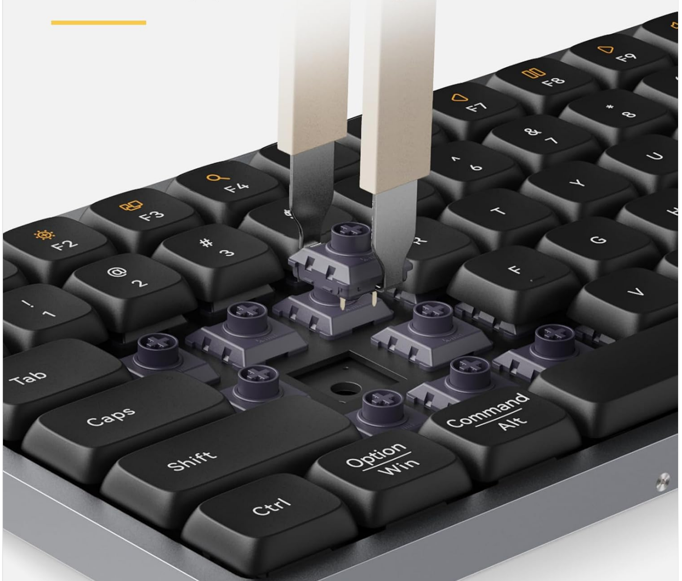
Image: Hot-swappable design allowing for easy switch replacement.
