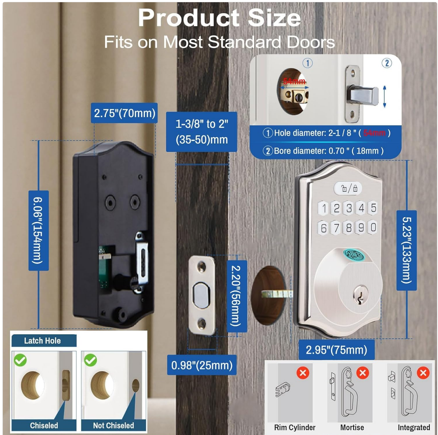
Figure 4.1: Detailed product dimensions and compatibility requirements for standard door preparation, including hole diameters and latch hole types.
