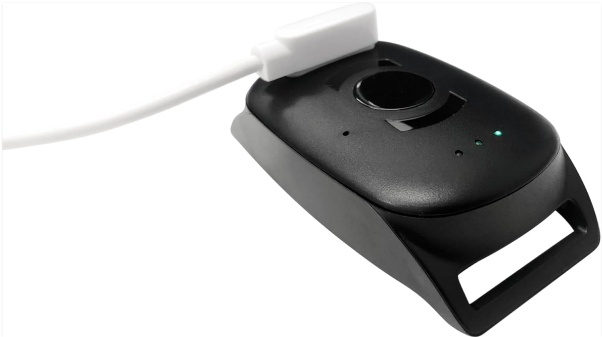
Figure 3: A MiniFinder Atto Pro GPS tracker actively charging, showing the magnetic cable connected and a green indicator light.
