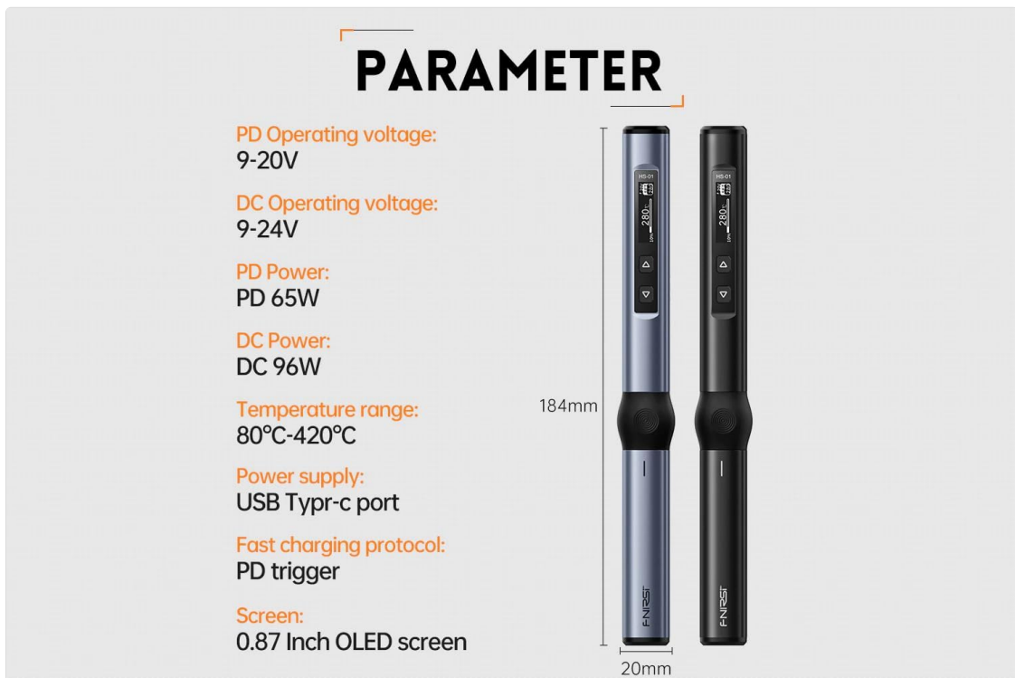
Image 5.1: Detailed parameters and dimensions of the FNIRSI HS-01 soldering iron, including PD/DC operating voltage, power, temperature range, power supply type, fast charging protocol, and screen size.
