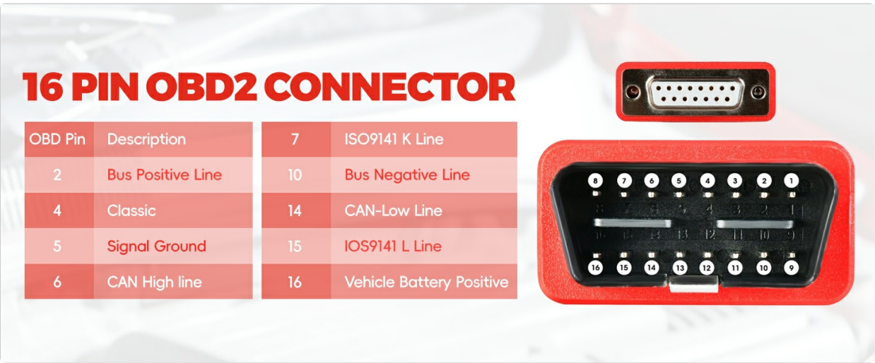
Image: Detailed diagram of the 16-pin OBD2 connector, illustrating the pin assignments and their descriptions.
