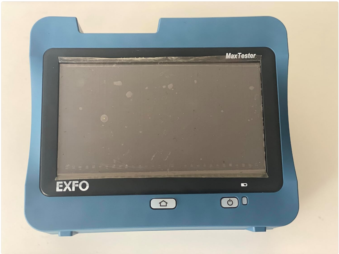
Figure 2.1: Front view of the EXFO Maxtester MAX-730D-SM1 OTDR module, showing the display and control buttons.
