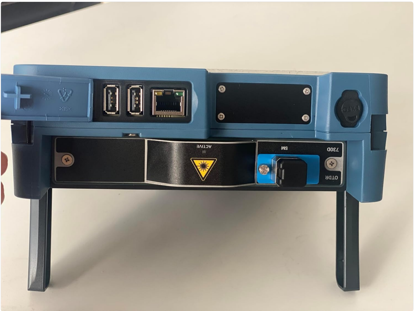
Figure 3.3: Side view of the EXFO Maxtester, illustrating the location of the USB ports and other connectivity options for data transfer.
