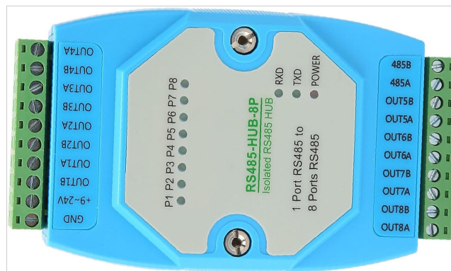
Figure 4: Top view of the RS485 hub, clearly showing the labeled terminal blocks for power input, master RS485, and the eight isolated slave RS485 outputs.
