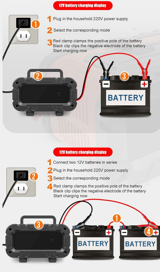
Image: Diagram illustrating simple connection steps for 12V and 24V batteries.
