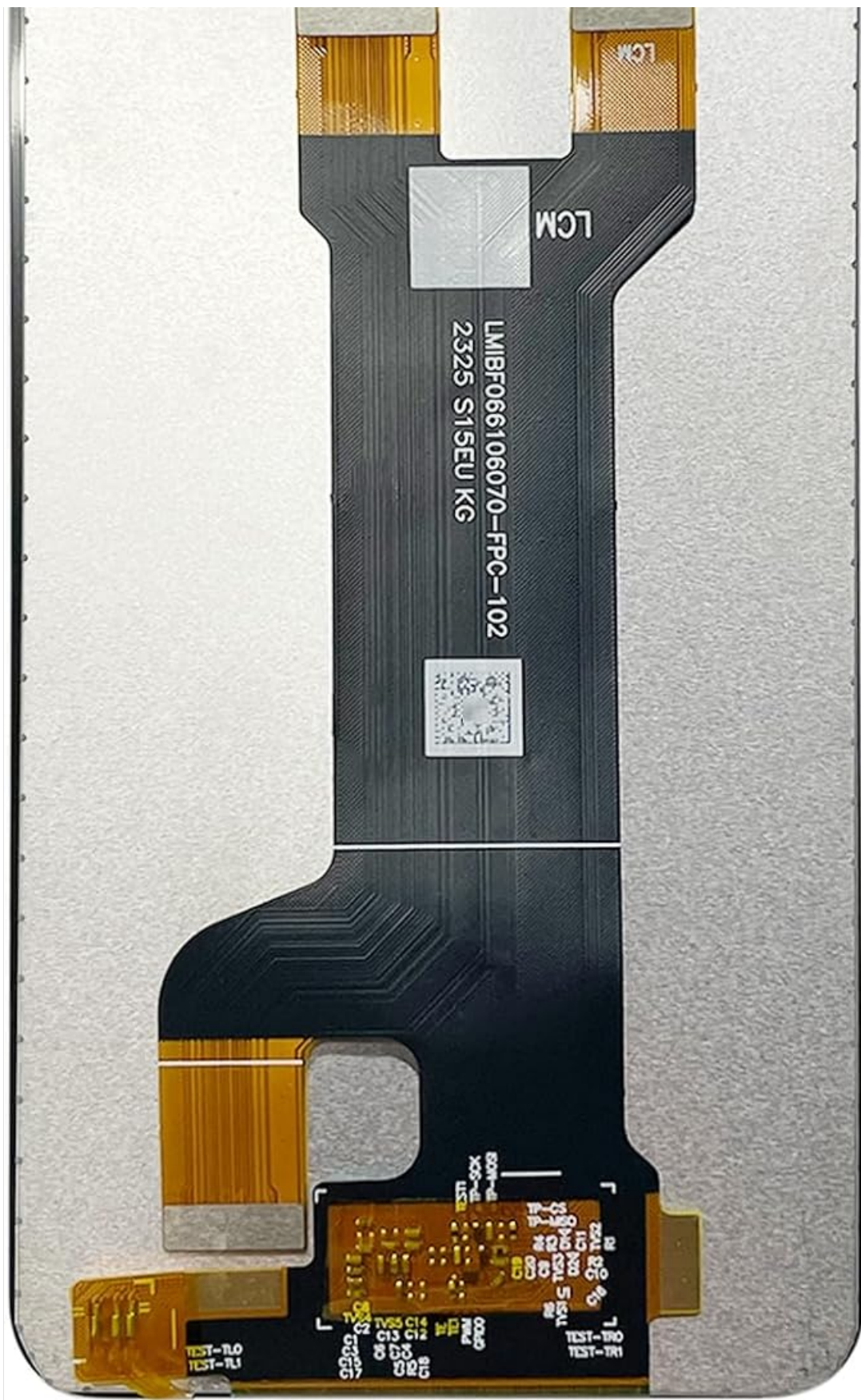
Image: A detailed view of the reverse side of the LCD screen assembly, highlighting the delicate flex cables and their connection points, which are crucial for proper testing and installation.
