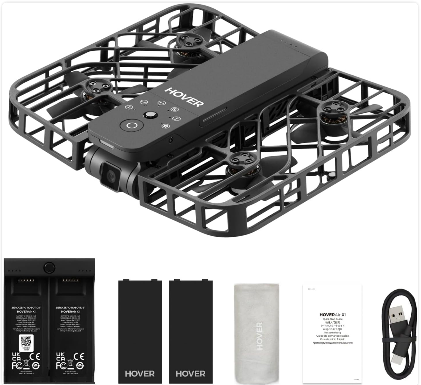
Image: The HOVERAir X1 drone in its unfolded state, alongside its accessories including two extra batteries, a charging hub, a storage bag, and a USB cable.
