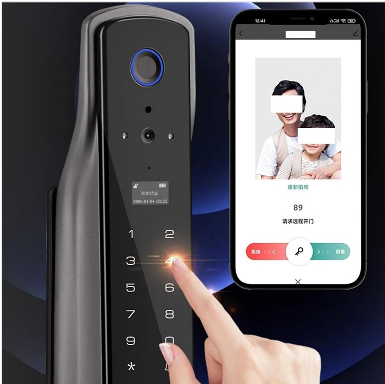
Image 5.2: Demonstrates unlocking the door using the keypad and receiving a notification or control option on the mobile application.
