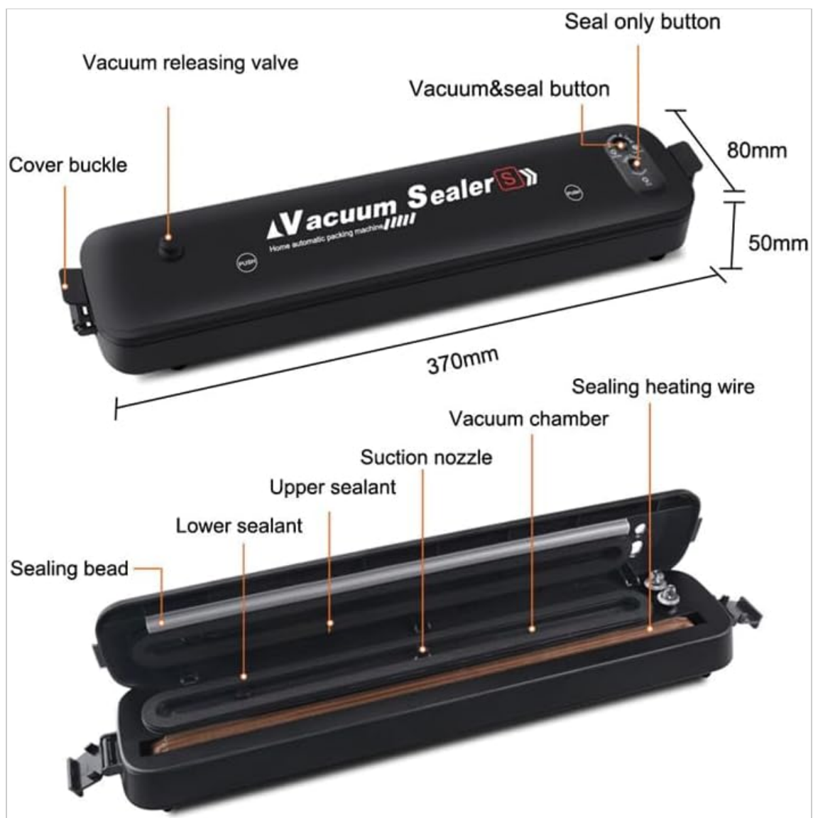
Figure 1: Labeled components of the vacuum sealer machine.
