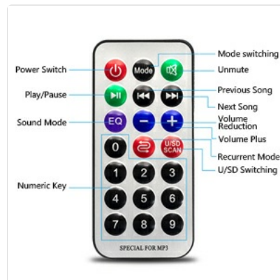
Image: A diagram illustrating the remote control and its various labeled buttons for different functions.
