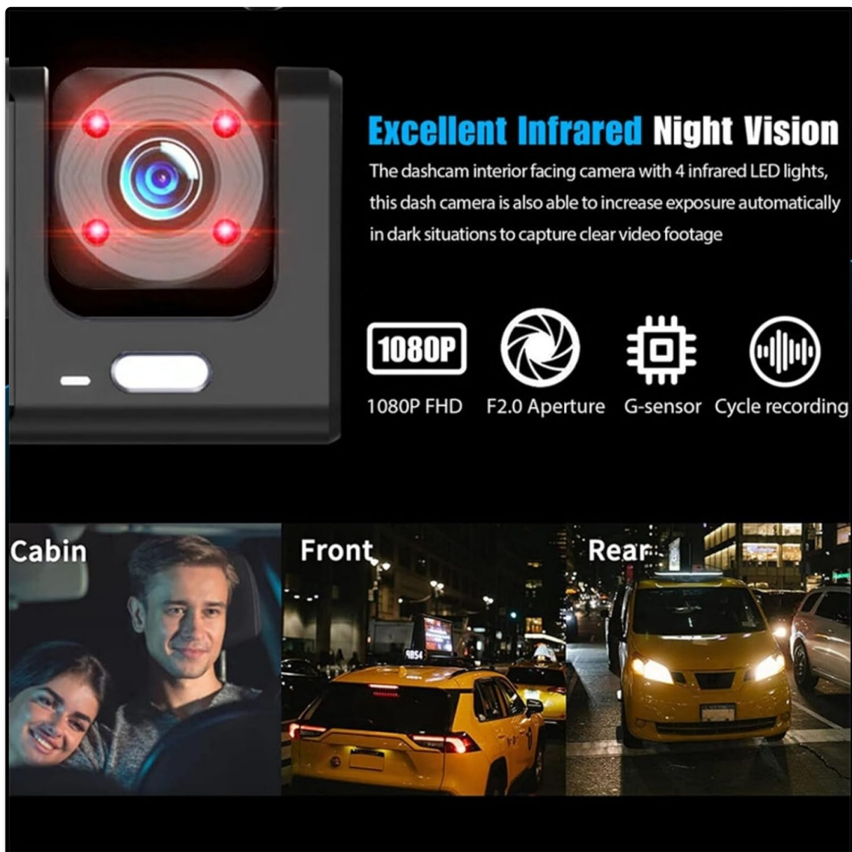
Image: The dash camera's interior-facing camera, highlighting its infrared night vision capability with four infrared LED lights for clear recording in dark environments.
