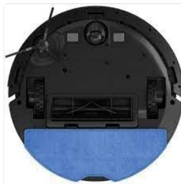
Figure 3.3: Bottom view of the Beko Robot Vacuum Cleaner, illustrating the main brush, side brushes, wheels, and the attached blue mopping pad.
