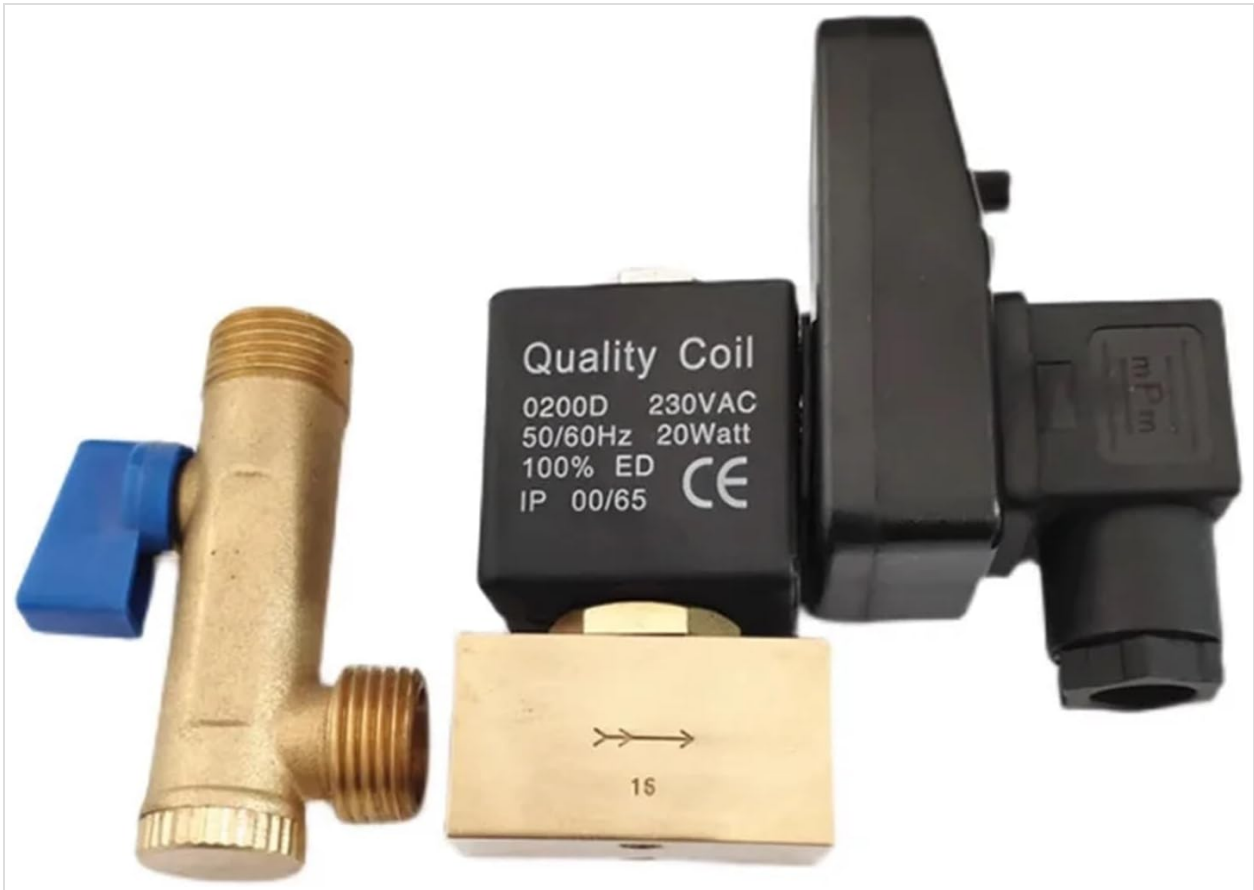
Figure 1: CONTIA 0200D Type A Electronic Timed Drain Valve. This image shows the main components of the Type A valve, including the solenoid coil, brass valve body, and a separate manual ball valve for isolation and manual draining.
