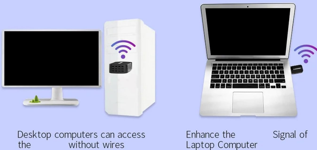
Image 4.2: Illustration of the dongle operating in Station Mode, allowing desktop and laptop computers to receive WiFi signals wirelessly.
