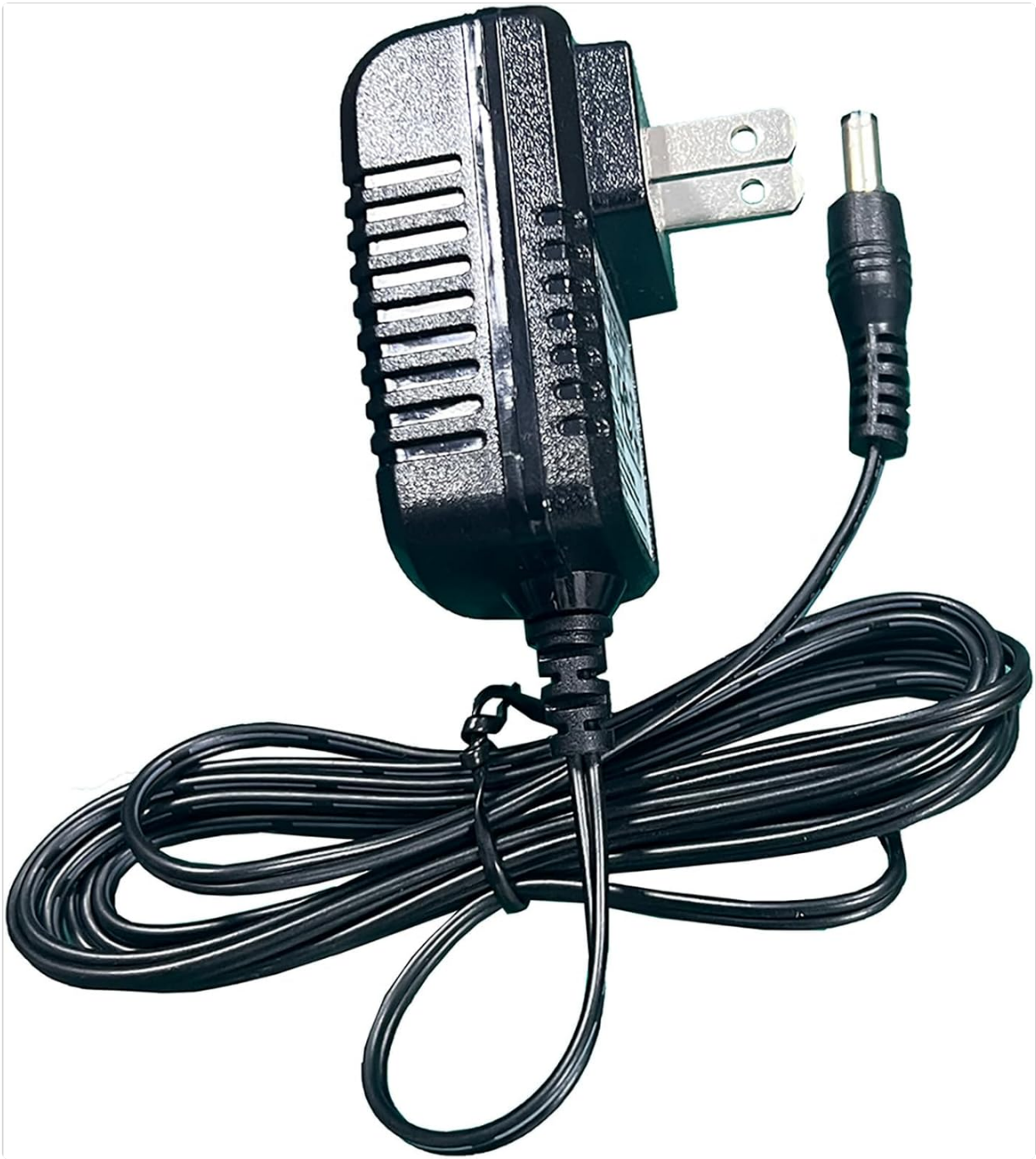
Image: The Heimerdinger 18V battery charger with its power cord and barrel connector. Input: 100-240V 50-60Hz, 0.8A. Output: 21V, 0.75A.
