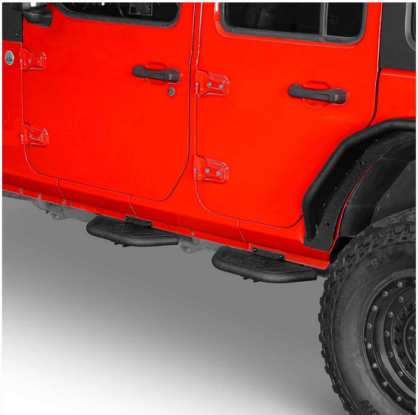
Figure 3.2: Side view of the running boards after successful installation on a Jeep.
