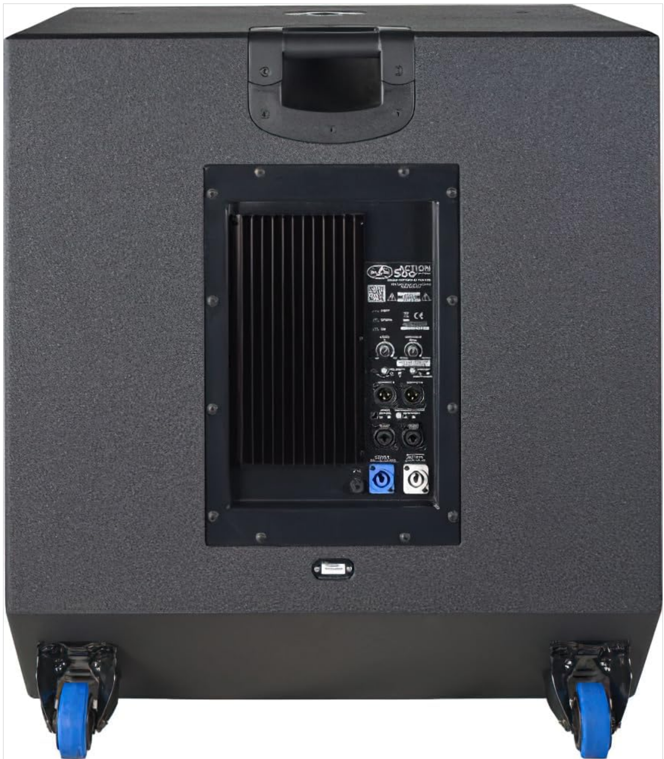
Figure 4.1: Rear panel of the ACTION-S118A-115 subwoofer. This view displays the amplifier module, including XLR input and loop-thru connectors, powerCON AC input and output, and control knobs for variable LPF and EQ settings.
