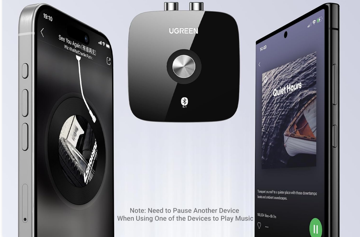
Figure 5: The adapter supports dual pairing for convenience.
