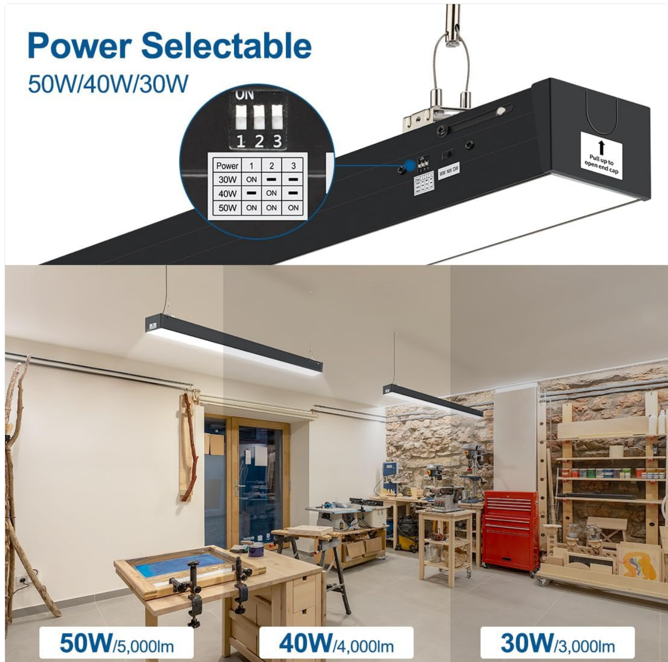
Figure 6: Power selectable switch (50W/40W/30W) and corresponding light levels.
