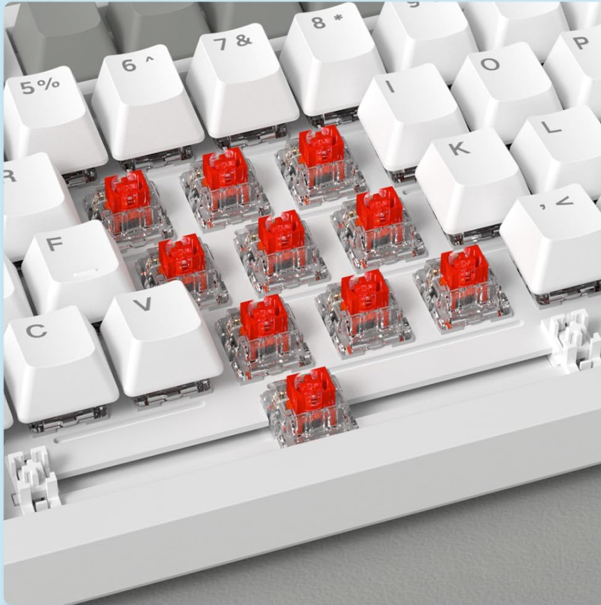
Figure 6: Illustration of the hot-swappable switch mechanism.
