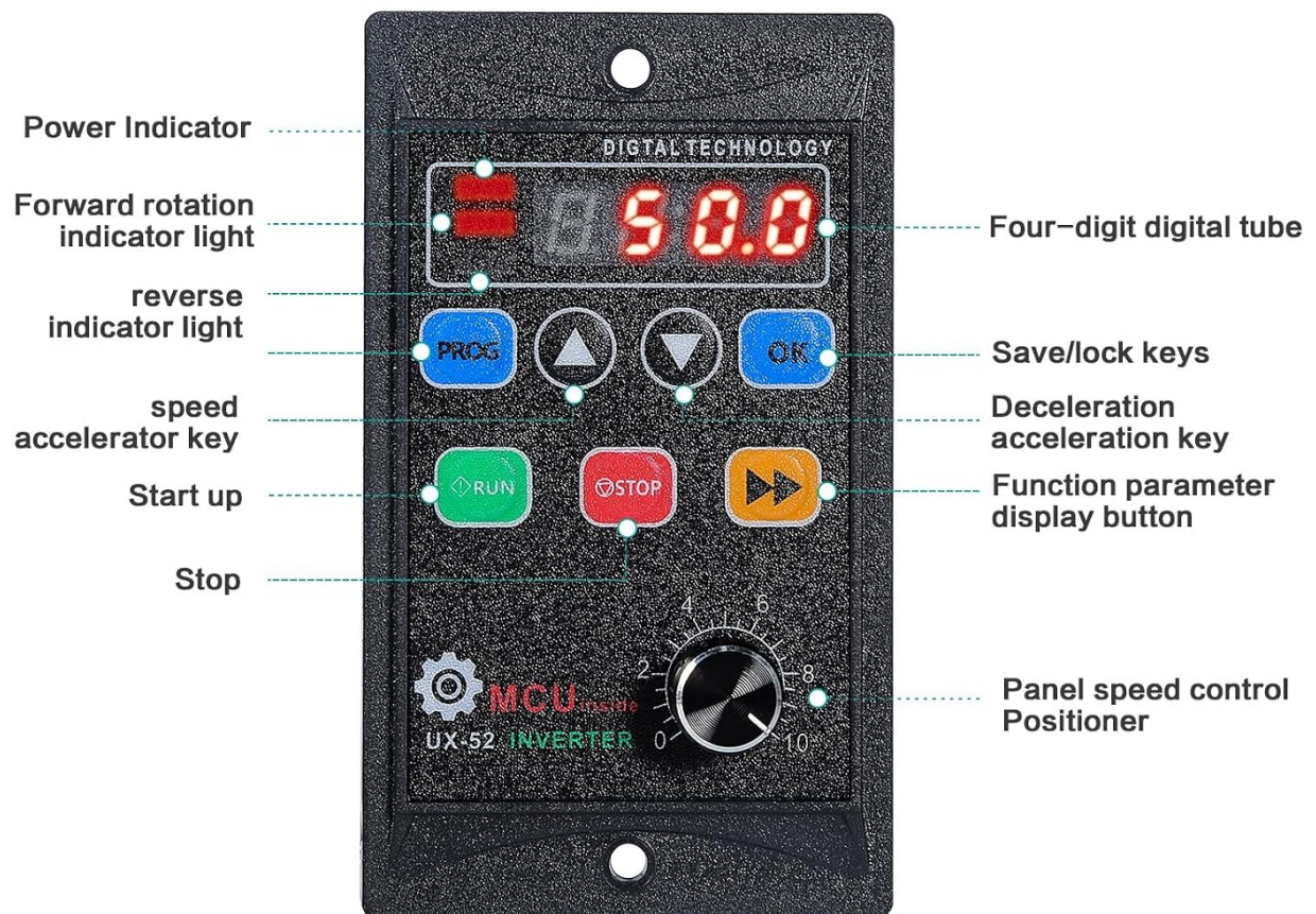
Image 3.1: VFD Operation Interface.
