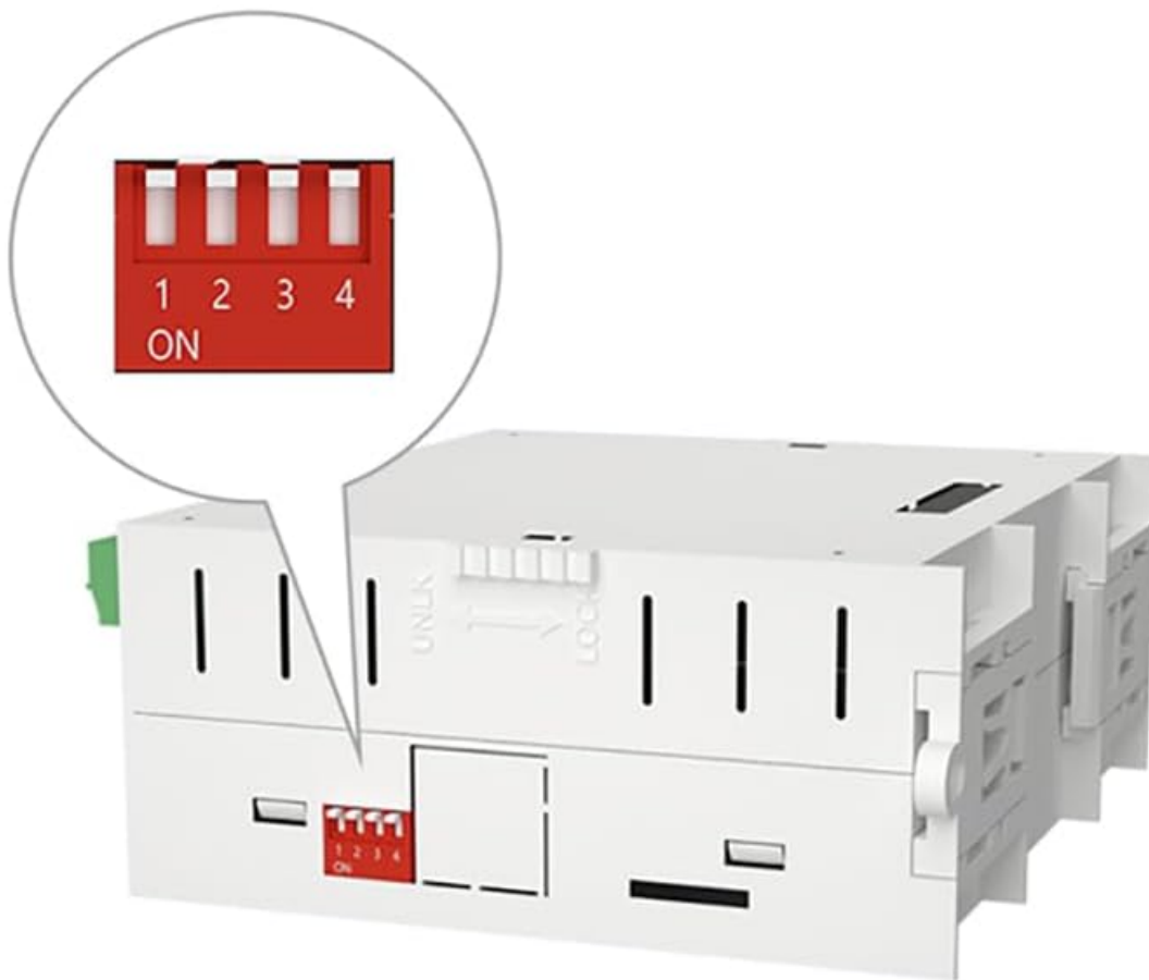
Figure 3.1: Image depicting the DIP switches on the EBYTE M31 module for quick Modbus address configuration without a host computer.
