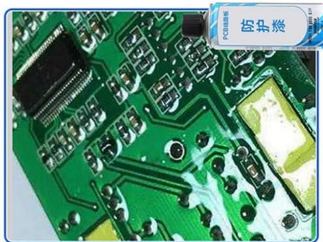
Figure 2.4: Image highlighting the module's robust design with anti-fungal, anti-humidity, and anti-salt spray properties, along with a close-up of its circuit board.
