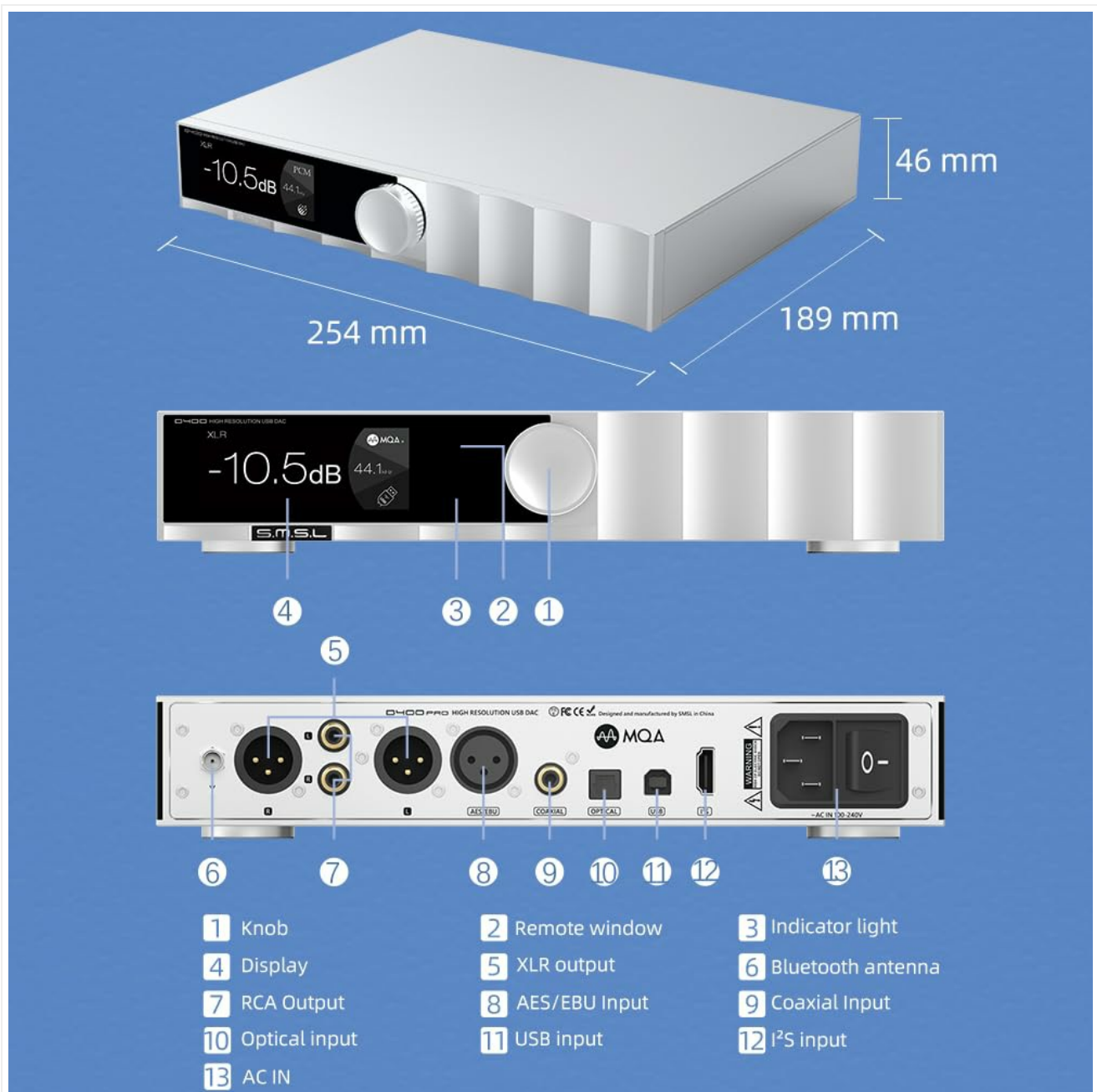
Figure 4.3: Detailed diagram of the S.M.S.L D400 PRO with labeled components and dimensions.
