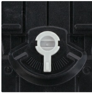
Image: A close-up view of the steering trim adjustment dial, typically found on the chassis of the RC car, used to fine-tune straight-line driving.
