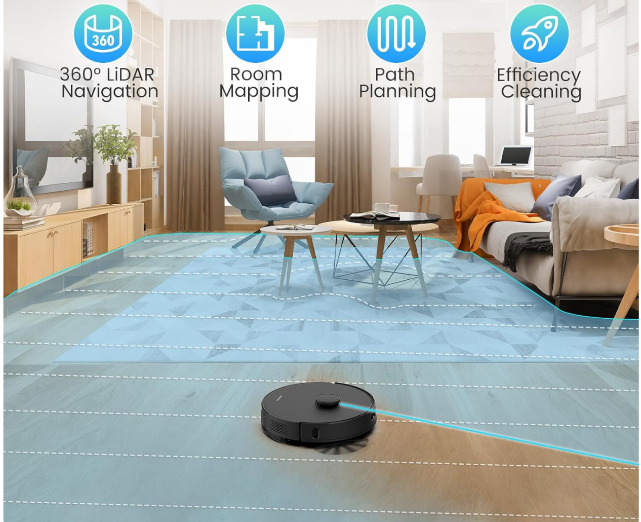
Figure 3: Visual representation of the robot's LiDAR navigation and mapping capabilities.
