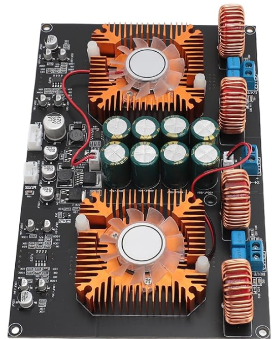
Image: An overhead view of the TPA3255 amplifier board, showing the layout of components, heat sinks, and connection points.
