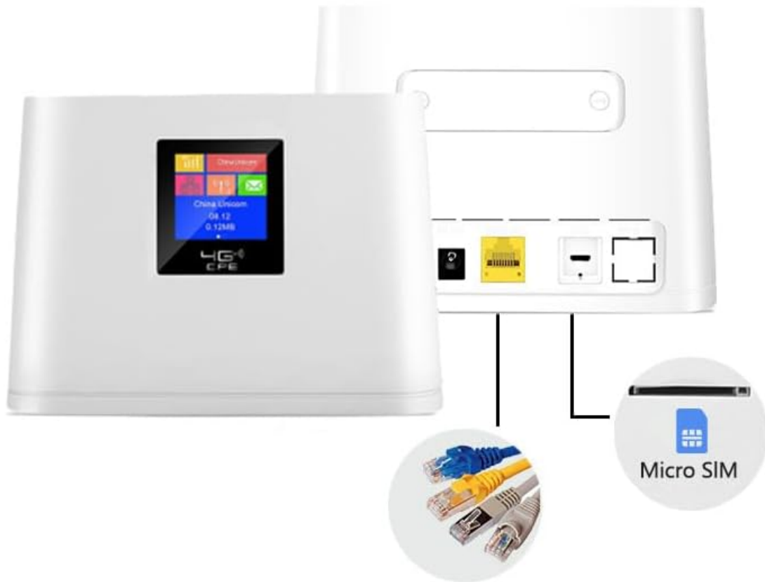
Figure 3: Rear view of the HOSAYA CPF908 Router, highlighting the RJ45 WAN/LAN port, dual power inputs, and Micro SIM card slot.
