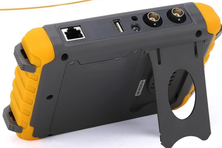
Image 4.2: Device protected by film and rubber, showing the kickstand and neck strap.
