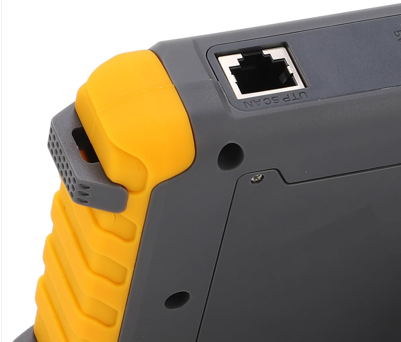
Image 6.1: Close-up view of the UTP SCAN port for network cable testing.
