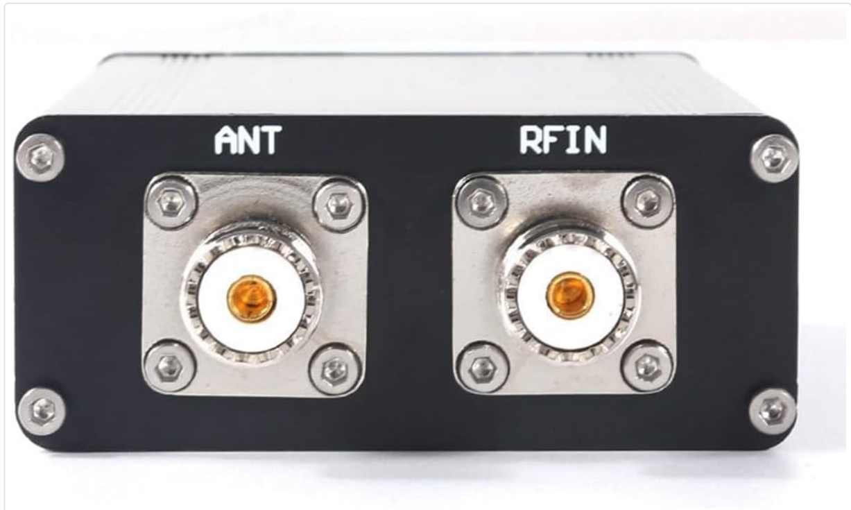
Figure 4.1: Rear panel of the ATU-100 Pro+ showing the ANT (Antenna) and RFIN (Radio Frequency Input) connectors.
