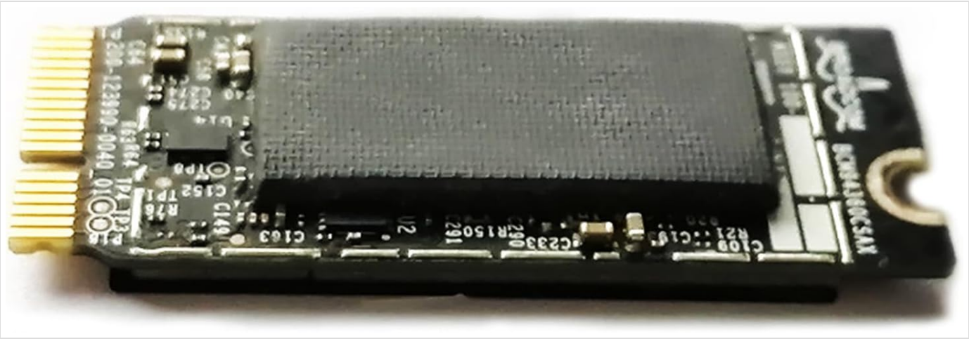
Image 4: Shows the reverse side of the Aokyitzm BCM94360CS/BCM94360CSAX Dual-Band Network Card, highlighting additional components and markings.
