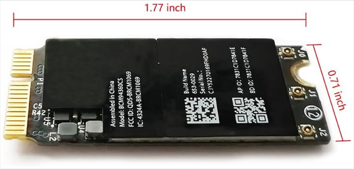
Image 3: Displays the physical dimensions of the Aokyitzm BCM94360CS/BCM94360CSAX Dual-Band Network Card, indicating its length and width.
