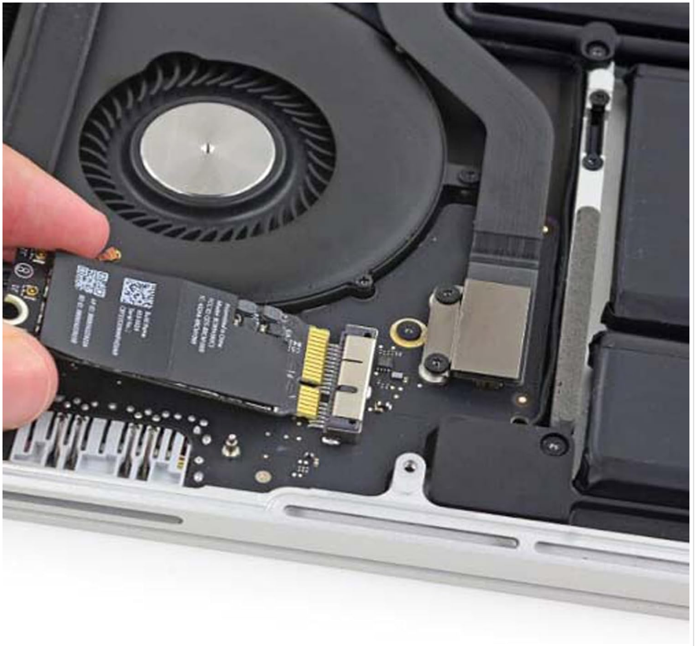
Image 1: Illustrates the installation of the Aokyitzm BCM94360CS/BCM94360CSAX Dual-Band Network Card into a compatible MacBook. The card is being carefully inserted into its designated slot on the logic board.
