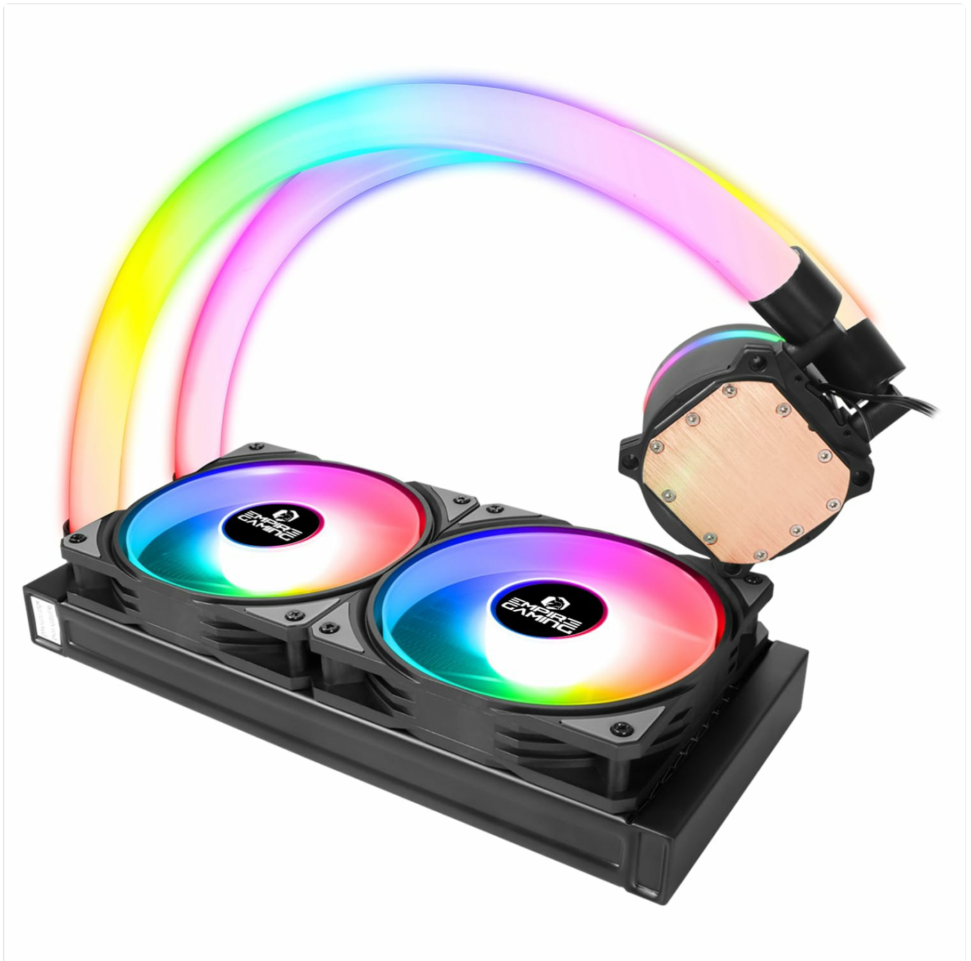
Image 5.1: Rear view of the pump and copper cold plate. This image shows the pre-applied thermal paste (if applicable) or the clean copper surface where thermal paste should be applied, and the mounting points for brackets.
