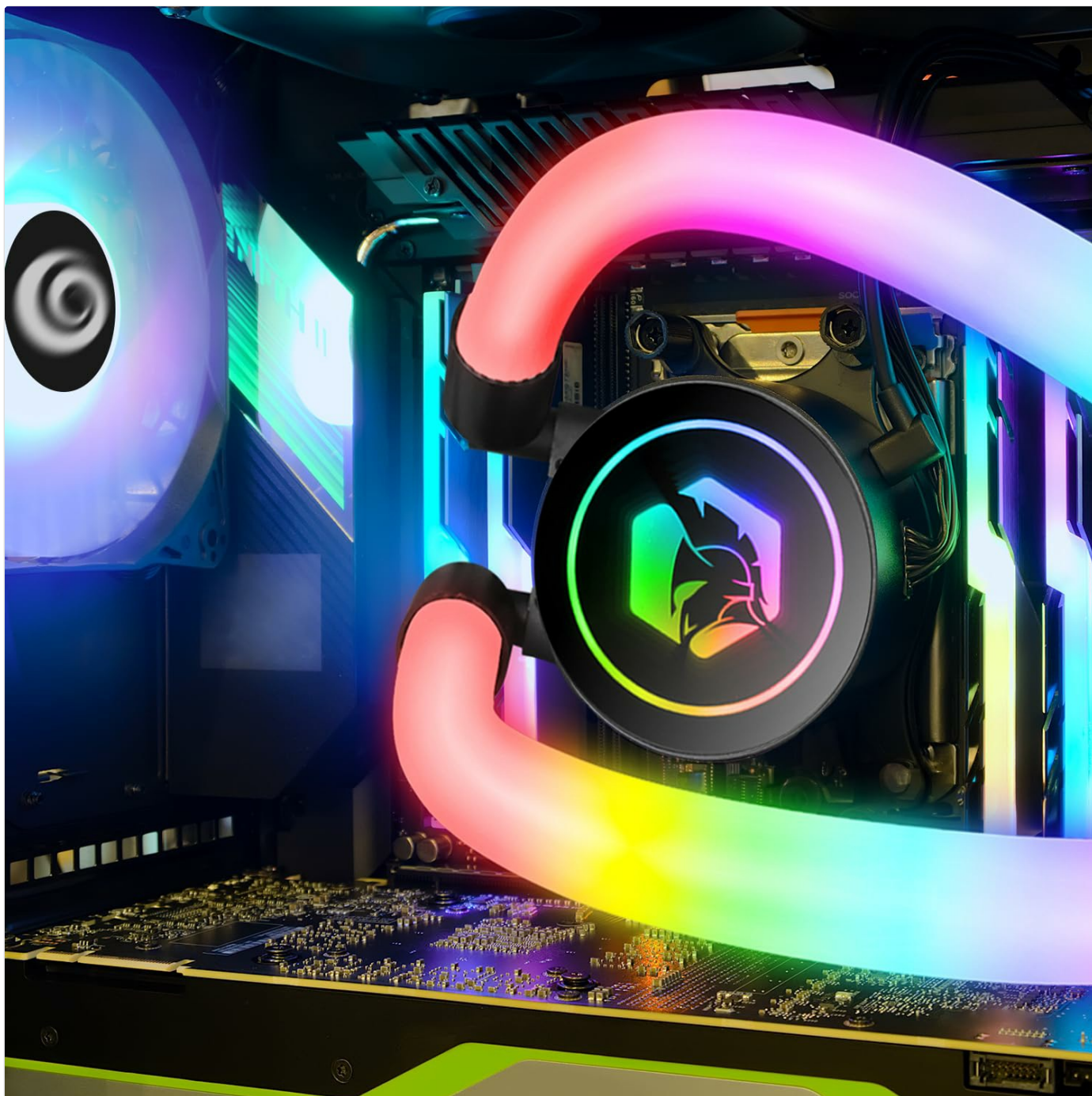
Image 5.2: AIO cooler installed in a PC. This image demonstrates the pump head mounted on the CPU, with the illuminated tubing and fans visible within a computer case.
