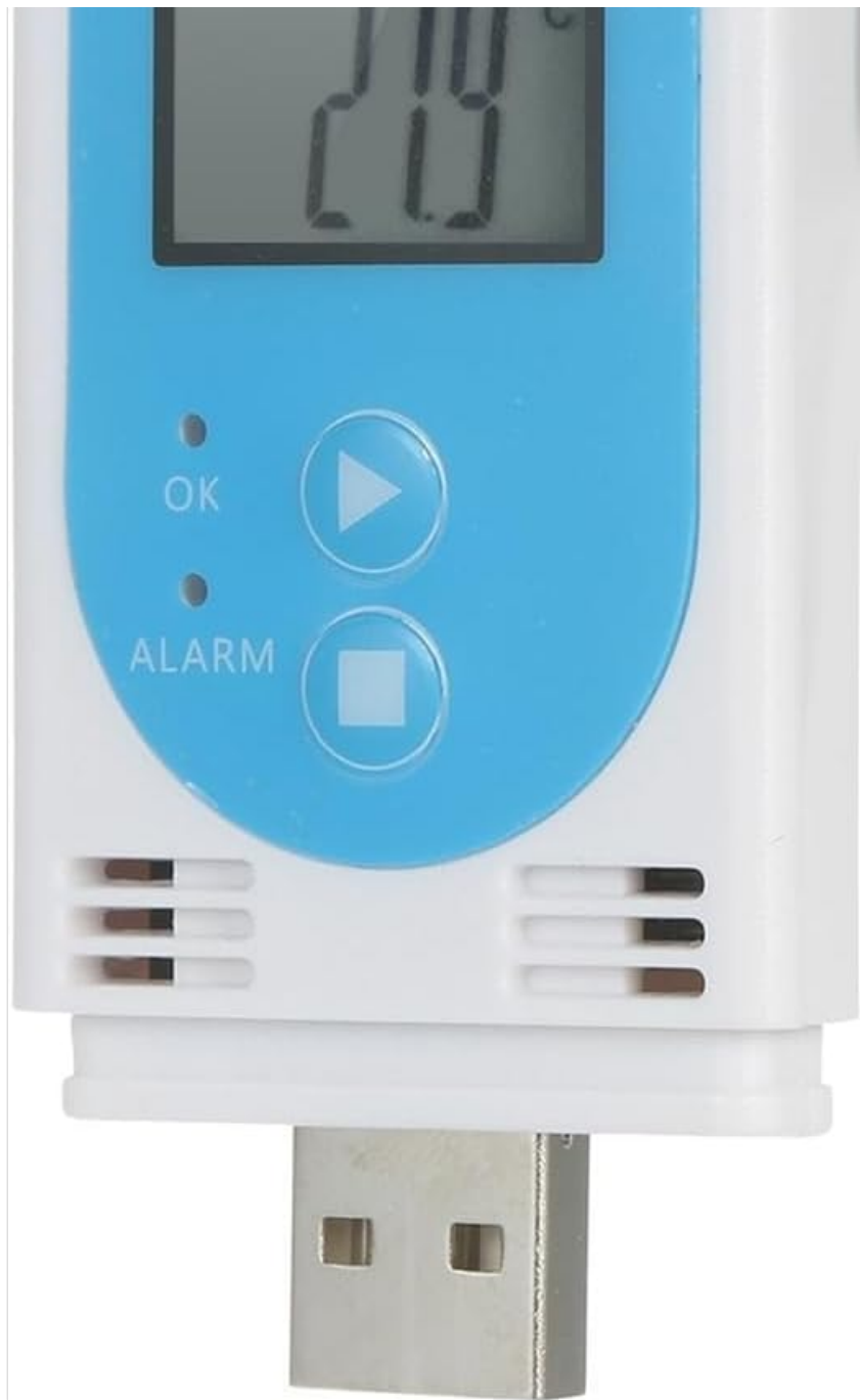
Figure 1: Front view of the Besuso TempU 03 data logger, showing the LCD display and control buttons.
