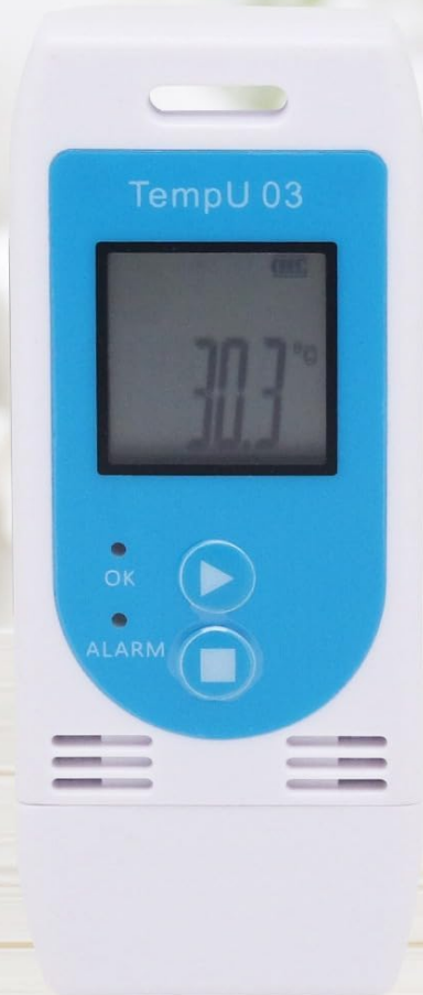
Figure 3: Diagram showing the LCD Display, Indicator Light (OK/ALARM), Start/Scroll/Mark Button, Stop Button, and Removable Case.
